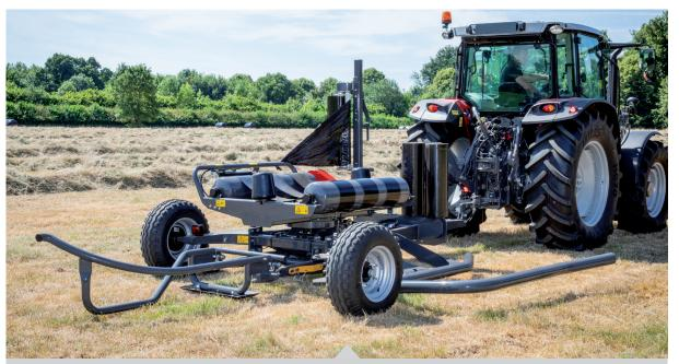
The MF TW 130 is a straightforward design wrapper with a grid frame, exceptionally low wrapping table and semi-automatic controls for fast and reliable trouble-free operation.
