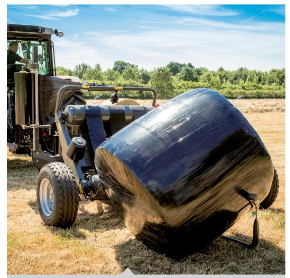
Bale discharge is exceptionally gentle, without the risk of damaging the film, thanks to a lowpositioned wrapping table which tilts close to the ground when unloading bales. An optional baler tipper is available to prevent the bales from rolling in hilly conditions, improving safety and reducing the time required for bale collections in the field.
